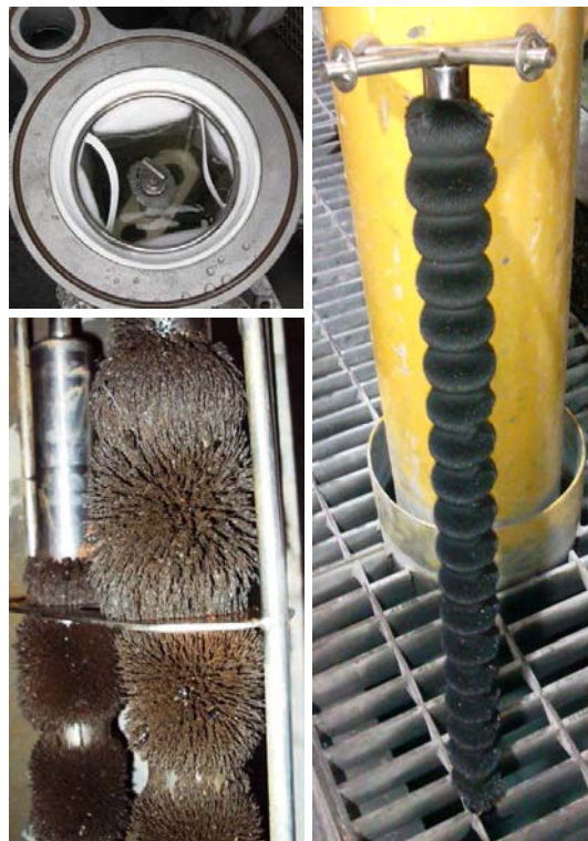
Top Left: Close up of saturated core. Bottom Left: Core tube assembly installed in P2 bag filter. Right: Standard P2 bag core tube saturated with ferrous material.
